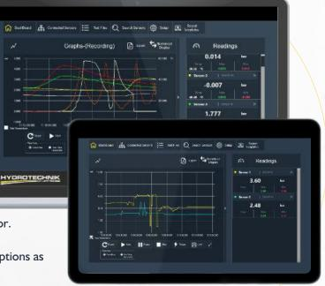
Data can be viewed in graphical or numerical format and recorded data can be exported in PDF or CSV format. During tests graphical data can be interrogated by zooming and also adding annotations.
