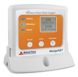
The RFPulse2000A is unique in that it not only calculates pulse count, but it also calculates pulse rate. Engineering units can be programmed into the device as a rate, which allows the device to calculate the measurement unit in rates per second, minute, hour or per day. This provides more useful statistics to the user when data logging over long periods of time.
