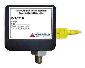
to 10,922 readings per channel. The storage medium is non-volatile solid state memory, providing maximum data security even if the battery becomes discharged. The PRTC210 can be started and stopped directly from your computer and its small size allows it to fit almost anywhere.
