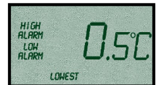
LCD displays the lowest recorded reading
