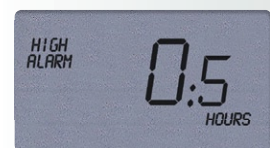
LCD displays the time above the specified high alarm setting for the current trip
