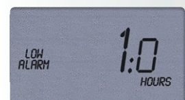
LCD displays the total time below the specified low alarm setting for the current trip
