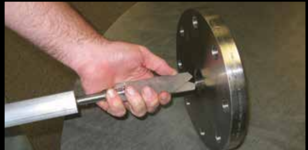
Squeeze the insertable paddle and guide it through the opening.
