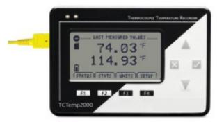
The **TCTemp2000** is a thermocouple temperature data logger perfect for applications requiring instant remote readings of temperature. The 8-button keypad and large LCD provide convenient access to current data and data logger setup. Additionally, memory and battery levels, external power status, sampling and recording status are shown on the LCD. This data logger has an internal temperature sensor and one external input for J, K, T, E, R, S, B or N type thermocouples.
